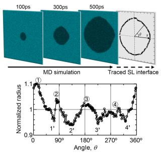
Fig. 1. Million-atom molecular dynamics simulation of spontaneous evolution of anisotropy in solid nucleus during solidification.<sup>52</sup> Results from Ref. 52 are reconstructed. (Top) Snapshots at 100, 300 and 500 ps and the trace of the solid–liquid interface obtained from the snapshot at 500 ps. (Bottom) Normalized radius of the solid nucleus as a function of rotation angle  $\theta$ .
