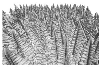
Fig. 7. Snapshot from a very-large-scale three-dimensional phase-field simulation of the directional solidification of a binary alloy polycrystal.<sup>35</sup> The calculation were carried out in a system with dimensions of  $3.072 \times 3.072 \times 3.072 \text{ mm}^3$  (4096 × 4096 × 4096 meshes) for a total time period of more than 100 s (4 million computational steps) using 768 GPUs with 768 CPUs on TSUBAME2.0.
