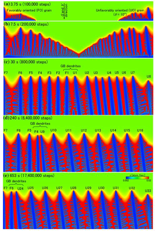
Fig. 5. Two-dimensional simulation of competitive growth of Al-3mass%Cu binary alloy bicrystal with  $V = 100 \ \mu$ m/s and  $G = 10 \ \text{K/mm}$ . The domain size was set to  $3.072 \times 1.152 \ \text{mm}^2$  (4096 × 1536 meshes) and the time step was  $\Delta t = 3.75 \times 10^{-5}$  s. Zero Neumann boundary conditions for  $\phi$  and u were set for all boundaries.
