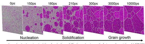
Fig. 2. Consecutive molecular dynamics simulation of nucleation, solidification and grain growth. An iron melt consisting of 1,037,880 atoms in a cell of 53.4  $\times$  53.4  $\times$  53.4  $\times$  4.3 nm<sup>3</sup> was isothermally undercooled at  $\Delta T = 1000$  K over 10,000 ps. Purple and white atoms represent iron atoms with and without the bcc configuration, respectively.
