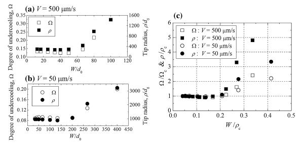
Fig. 3. Convergence behavior of degree of undercooling and curvature radius of the dendrite tip during directional dendritic growth in Al-2mass%Cu alloy calculated for (a) V = 500 and (b) 50  $\mu$ m/s. (c) Convergence behavior plotted on normalized axes.
